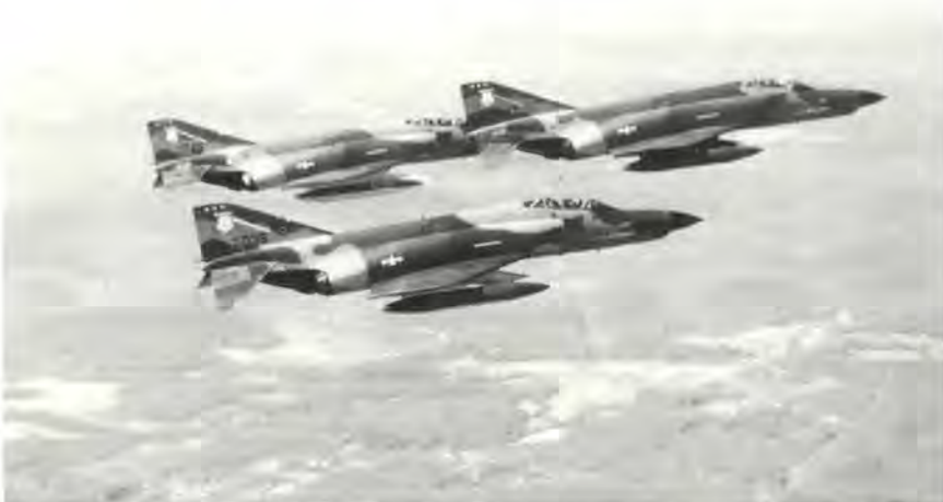
With or without leading edge slats, the F-4 is very sensitive to lateral asymmetry, aft CG, pitch rate, and yaw-roll coupling.
