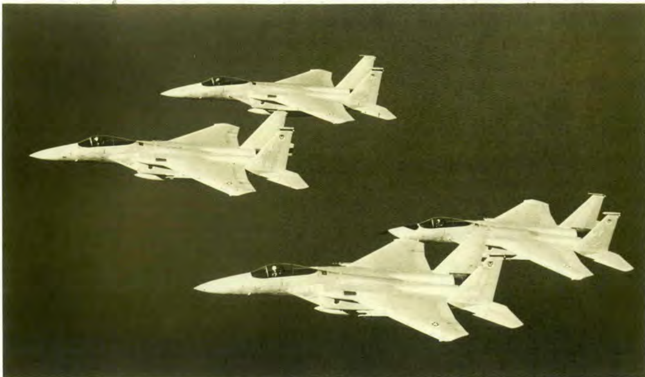
Tests have shown that the airplane is self recoverable in air-to-air configurations if controls are neutralized when the spin warning tone comes on.
